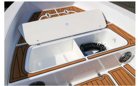
The live bait tank is baffled
