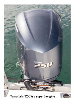
with a 200hp four stroke and can tell you it goes well, but there's no doubt a 250 will provide the ultimate in performance. Pacific Marine had fitted the test boat with a new Yamaha F250, which is up there with the best V6s you can buy. It's a 4.2 litre, V6 engine that weighs in at 254kg, which is 26 kilos under Signature's maximum transom weight.
